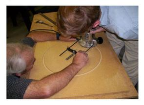
2.) use tools (router and or jigsaw) to carefully cut out a perfect circle 16 3/8" .. After the hole is cut you can sand down the inside edges to make it even smoother so your disc will turn smoothly.
