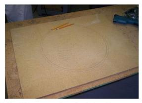
1.) Carefully measure lines for hole to be cut 16 3/8" "Measure twice, cut once" .This photo shows it centered. Personally, I'd make it offset a bit, to leave room on the side for Ex-sheet. See the plans by Jim MacCauley included in this pamphlet.
