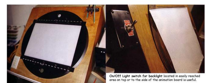
One other customizable option that is nice to have with any style of animation desk is an On/Off switch located in an easy to reach area on the top or to the side of the desk area, so you can switch the backlight on and off without fumbling for the switch on the cord underneath the table. An alternative would be to use a foot switch to switch the backlight on and off by simply clicking on the switch with your foot.
